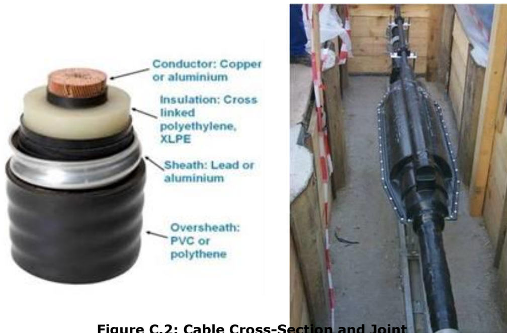
Figure C.2: Cable Cross-Section and Joint
